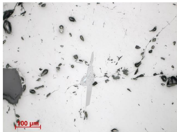
Figure 6.9 Left: Massive magnetite (white), hematite (lighter) and ilmenite (darker) occur as fissure filling (RL PPL). Right: Massive magnetite grain (white) with ilmenite (grey) developed at a fissure (RL PPL).
